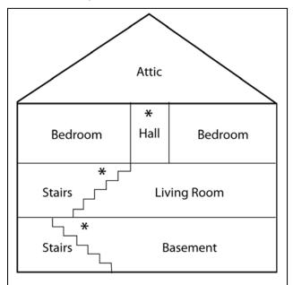
Install a smoke alarm and a carbon monoxide alarm (or combination alarms) in the basement and on each floor except the attic or a storage area.
