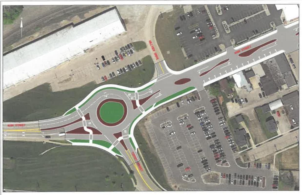
As shown on Table 12, the dual westbound lane roundabout design is expected to allow all traffic movements to operate at LOS 'C' or better during both the morning and evening peak hour time periods.
