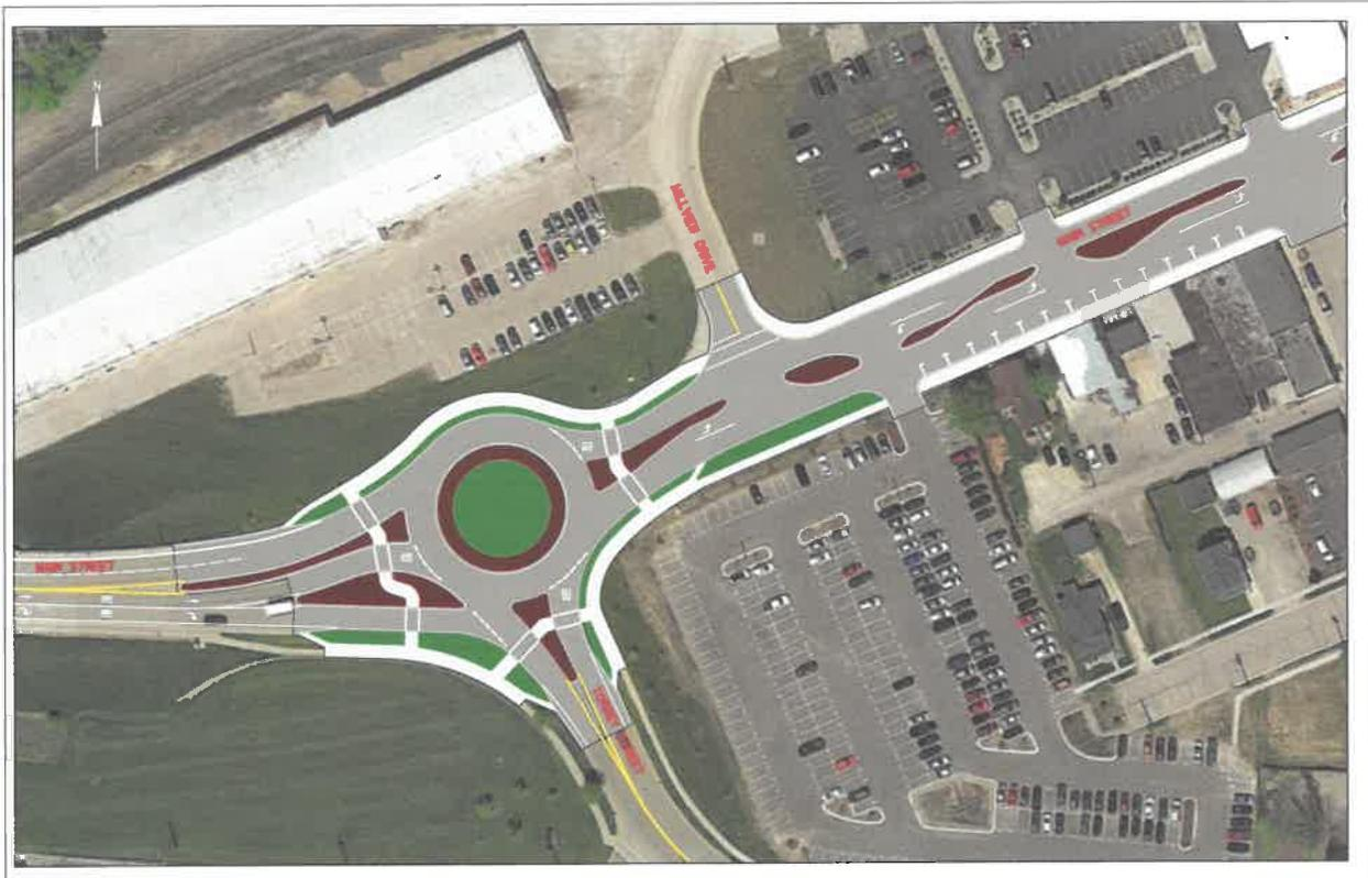
Table 10 summarizes the operational traffic improvement associated with construction of a single-lane roundabout at the Torrey Street intersection with Main Street. The design is
