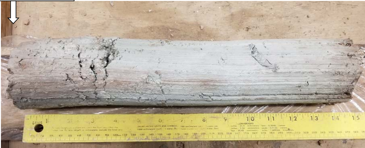
Figure 2 – Photograph of Boring B4-18 sample 4, from 6 to 8 feet below ground surface (EL. 739.12 to 737.12 +/-).
