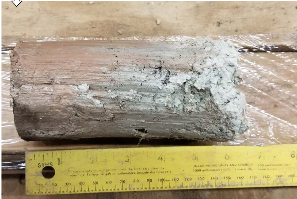
Figure 1 – Photograph of Boring B4-18 sample 2, from 2 to 4 feet below ground surface (EL. 743.12 to 741.12 +/-).
