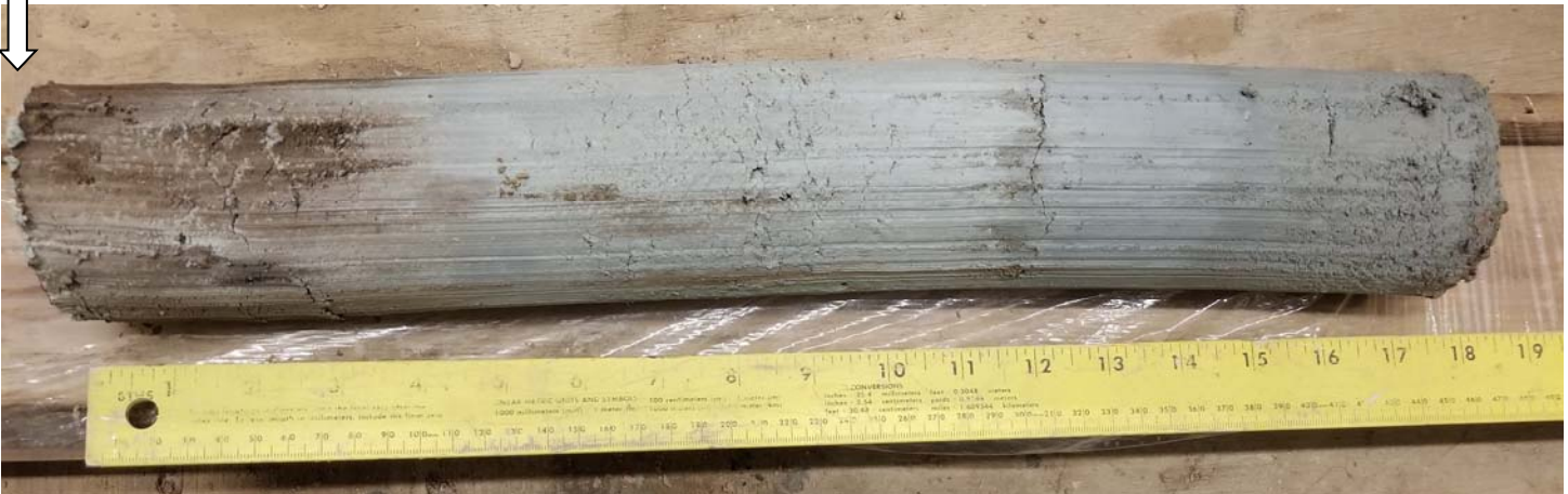
Figure 4 – Photograph of Boring B9-18 sample 6, from 11 to 13 feet below ground surface (EL. 738.86 to 736.86 +/-).
